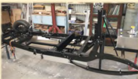
The chassis well under way with front axle and springs fitted and structure to support the body
