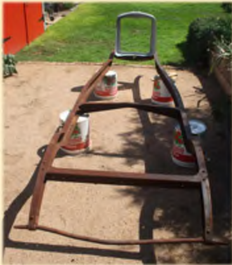
The bare FIAT 501C chassis and radiator shell
