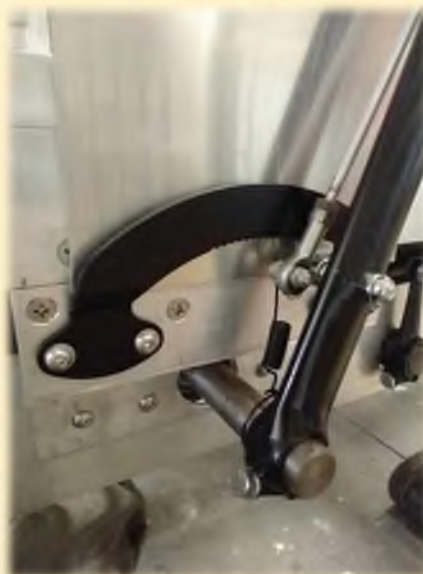
Handbrake lever is a combination of the top section of the original 1924 Fiat lever and Model T
