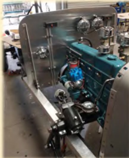
Engine fitted along with firewall and steering box
