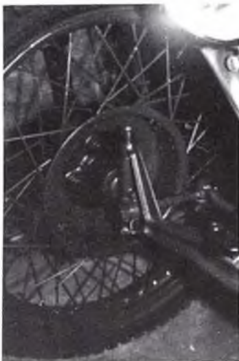
Above: Absolute simplicity, front axle without the complication of messy things such as brakes
