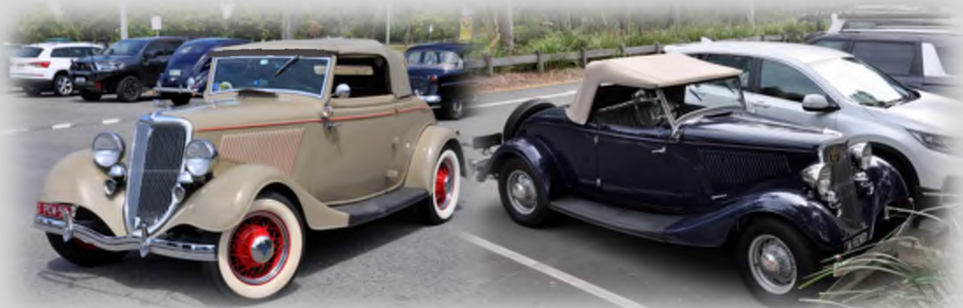
Here are two pictures comparing the 1934 Roadster and Cabriolet. While they are both single seaters, the Roadster has a detachable windscreen and side curtains. The Cabriolet has a fixed windscreen and wind-up windows. Trevor Poulsen
