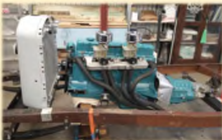
Trial fitting of the 3.3 litre Holden engine into chassis
