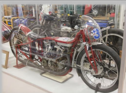
The world's fastest Indian motorcycle is Burt Munro's modified 1920 Indian Scout 953cc, which set a land speed record of 184.087 mph at the Bonneville Salt Flats in 1967 (two ways) on display at Invercargill
