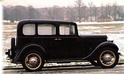
the first mass produced car to have full synchromesh transmission. It was the ten horse power model with a 30bhp 1.2 litre side valve four cylinder engine, still with cable brakes.
