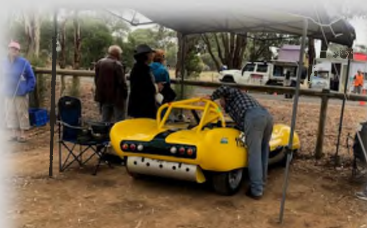
Replicas of the famous Lotus 11s are often seen in historic motor sport. Chris Dingle's is a fibre glass replica which he built up himself has a modified Austin Healy Sprite 1300cc engine. 17.2 secs
