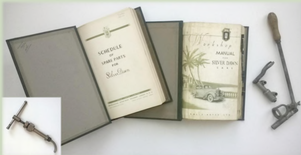
Useful manuals and special tools for the garage but not supplied with each car when new. The long tool is for removing inlet valve springs in situ and (left inset) is its companion which threads into the spark plug holes; the L shaped tool is for extracting the exhaust valve springs.
