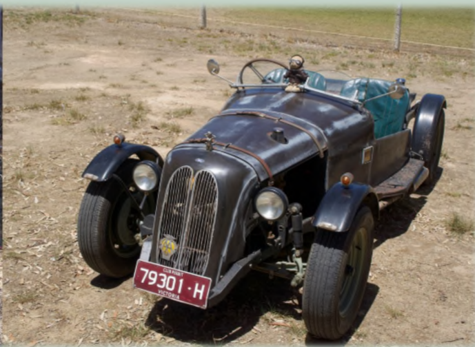
The 1953 Dellow Mk III, using Ford Prefect components to compete in post-war mud trials
