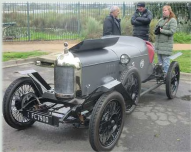
An outstanding restoration by Matt Spoljarevik, a replica of the earliest MGs ever produced – a 1925 MG of obvious Morris Bullnose descent. Notice the “Sloper” carburettor forerunner of the SU we are familiar with and the Hotchkiss engine from the factory that Morris took over in England after WWI.
