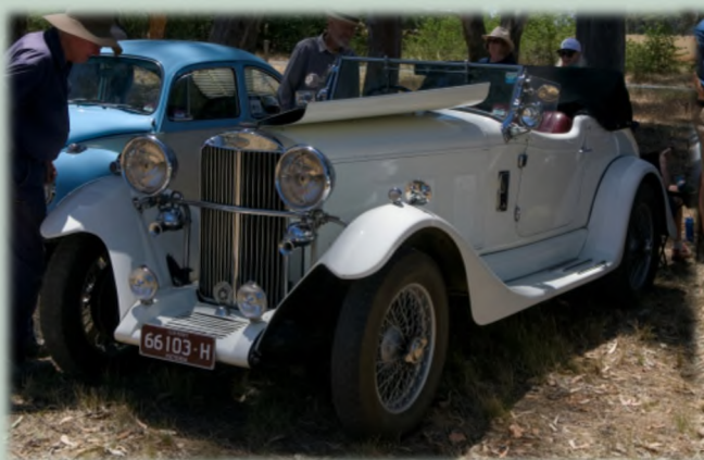
Brian Canny's 1933 Sunbeam Speed 20, with a 3.4-litre Jaguar engine under the bonnet
