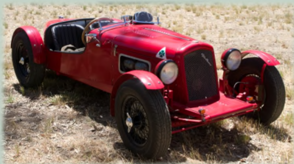
John Davey's Special: a 1936 Triumph Gloria chassis paired with an Alfa 104 engine
