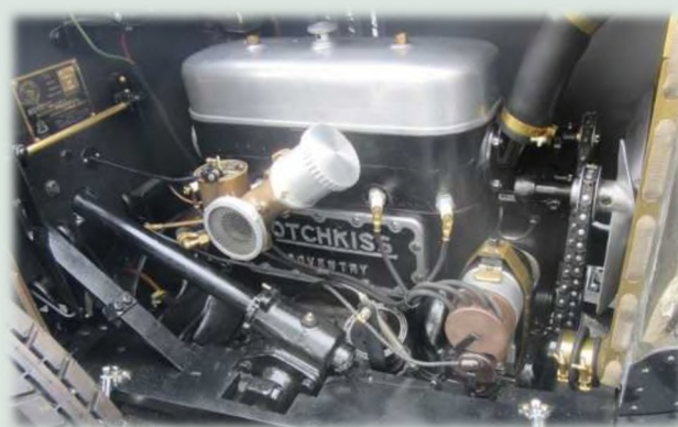
An outstanding restoration by Matt Spoljarevik, a replica of the earliest MGs ever produced – a 1925 MG of obvious Morris Bullnose descent. Notice the “Sloper” carburettor forerunner of the SU we are familiar with and the Hotchkiss engine from the factory that Morris took over in England after WWI.
