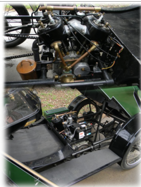
9hp V twin engine Riley
