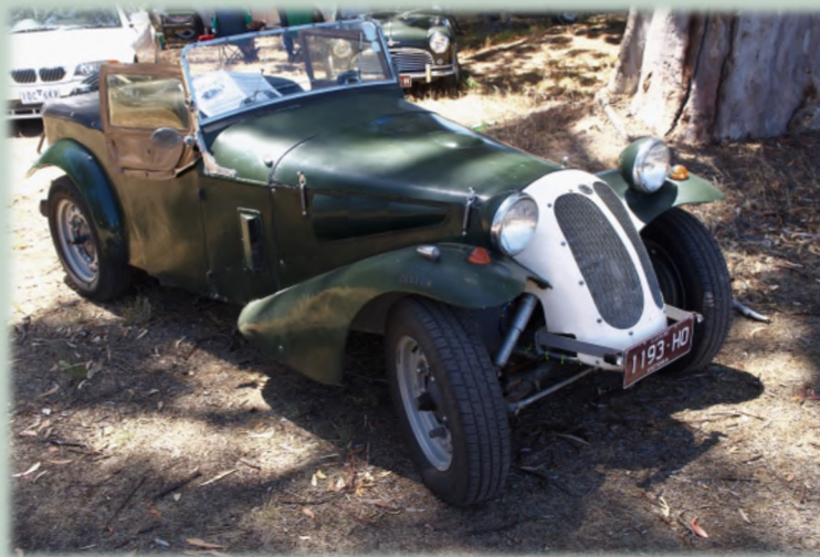
The 1953 Dellow Mk III, using Ford Prefect components to compete in post-war mud trials
