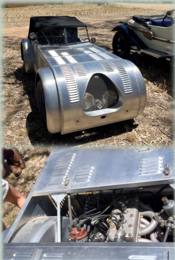
Bodied by Steve Barnett of Harcourt, his 'Tank' Austin Seven. The body style is based on the Type 32 "Tank de Tours Bugatti". Named for resembling the tanks of WWI that ran in the 1923 French Grand Prix at the Tours circuit in France. The Austin 7 was previously Max Foster's Austin 7 racing car.
