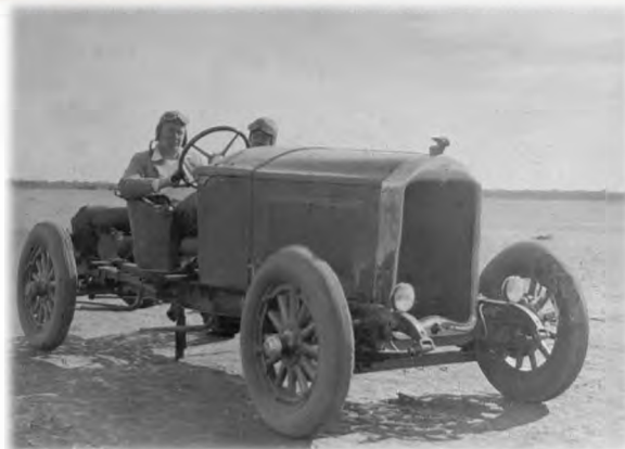
1928 Lake Perkolilli Buick This Buick was an impressive looking car. It appeared to have been based on a Buick Standard Six built between 1925 and 1927, with more 1927 than earlier parts. It had the wire wheels, which were an option at that time and the 12 inch mechanical brakes.
